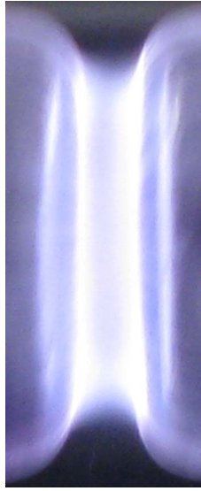
Fig. 2. Photograph of the plasma. Applied voltage: 6 kV. Pulwidth: 999.4 \mu\text{s} . Pulse repetition rate: 1 kHz. Ar flow rate: 200 sccm.
