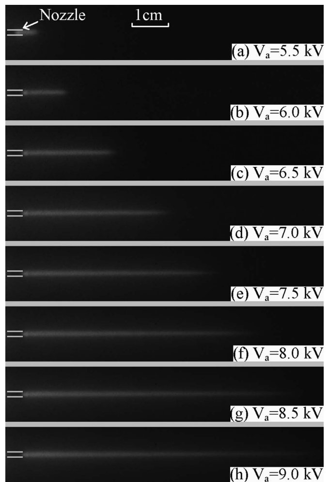
FIG. 2. Photographs of the plasma for different applied voltage V_a . Pulse width t_{pw}=800 ns, pulse frequency f=4 kHz, and He flow rate q=0.5 l/min. Glass tube is attached to the nozzle.
